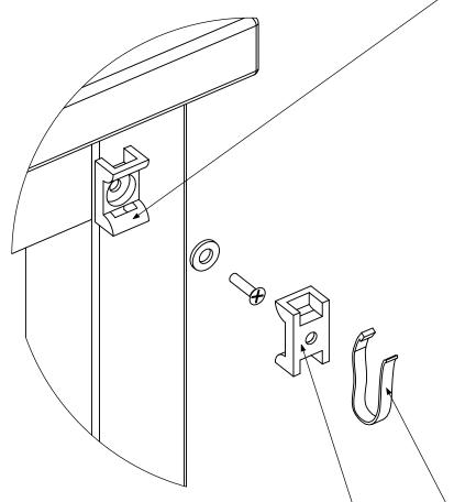
2 Step. Attach the 2nd plastic block to the wall. Own screws required.
