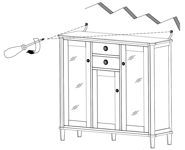
Always ensure that the wall attachment strap is correctly fitted.
